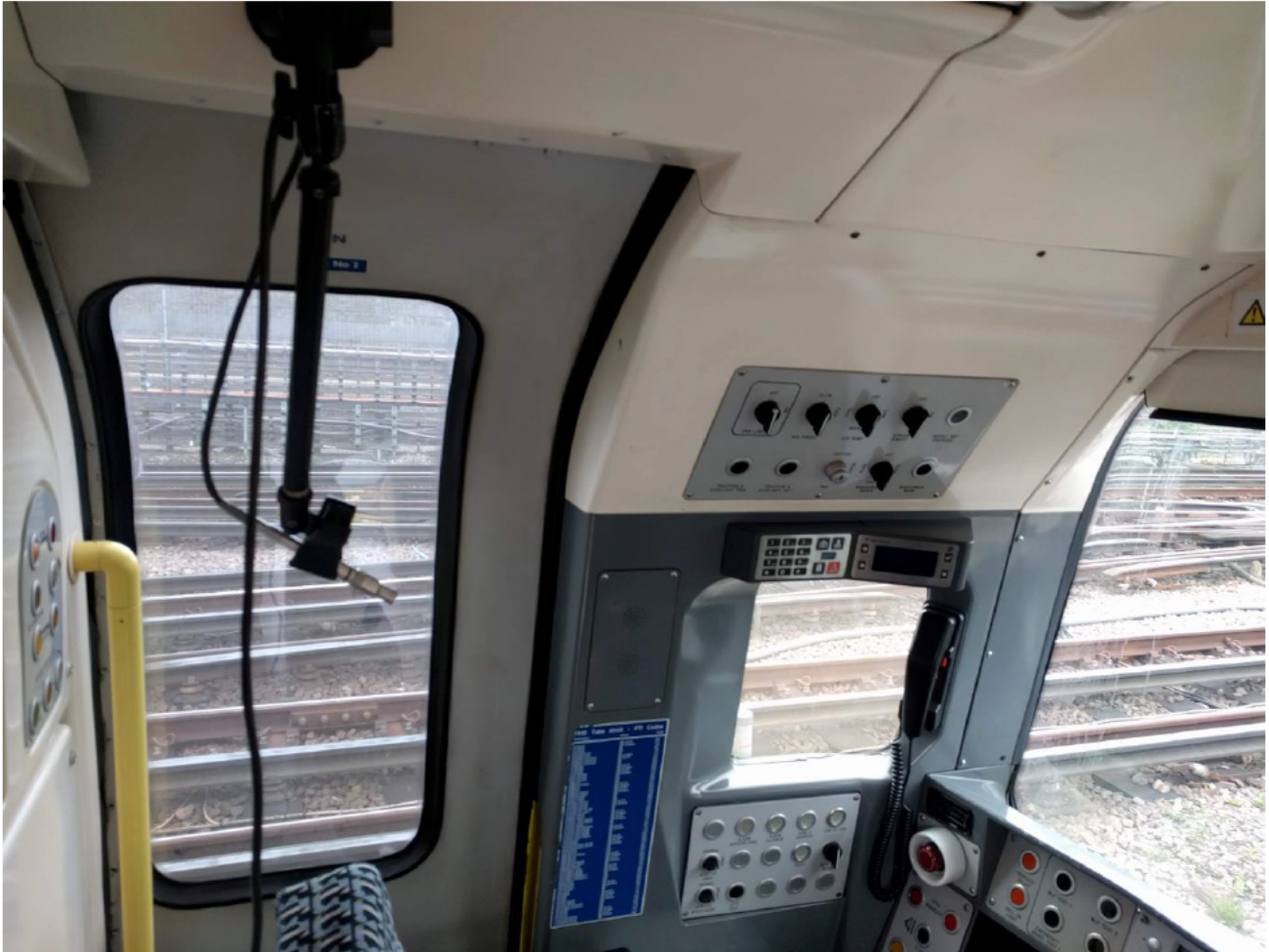
Figure C1 - Northern line 1995 tube stock cab and microphone arrangement
